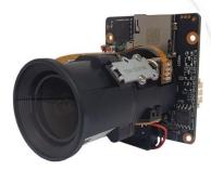
The IM30Z33W-5X 3 MP 5x WIFI module It is based on the HiSilicon embedded coding platform and adopts a 1/2.8 "low illumination 5 million CMOS image sensor, which has good low illumination effect and wide dynamic effect, and the maximum output resolution can reach 2304X1296@20fps The image is clearer and more delicate. Suitable for scenes that require high-definition image effects.
