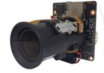
The IM50Z35W-5X 5 million 5x WIFI module It is based on the HiSilicon embedded coding platform and adopts a 1/2.8 "low illumination 5 million CMOS image sensor, which has good low illumination effect and wide dynamic effect, and the maximum output resolution can reach 2592X1944@20fps The image is clearer and more delicate. Suitable for scenes that require high-definition image effects.
