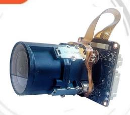
The IM30S07 3MP 10X automatic zoom high-definition network module is based on the Goke embedded encoding platform, using a 1/2.8 "low illumination 3MP CMOS image sensor, with good low illumination and wide dynamic effects, and a maximum output resolution of up to 2304X1296@20fps The image is clearer and more delicate. Suitable for scenes that require high-definition image effects.
