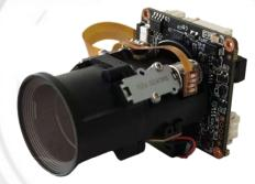
The IM20A01W-5X is a cost-effective 2MP surveillance network camera module designed for both indoor and outdoor use. It features a 1/2.8" Sony IMX307 STARVIS sensor and is powered by the GOKE GK7205V200 SoC, equipped with 512Mb of RAM.It Supports 2.4G WiFi and RJ45 Network Connectivity. In terms of extended I/O capabilities, it supports dual light source illumination, as well as microphone and speaker connections, enabling two-way audio and additional interfaces.
