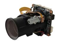
The IM20A03-5X is a cost-effective 2MP surveillance network camera module designed for both indoor and outdoor use. It features a 1/2.8" Sony IMX307 STARVIS sensor and is powered by the GOKE GK7205V300 SoC, equipped with 1Gb of RAM. In terms of extended I/O capabilities, it supports dual light source illumination, as well as microphone and speaker connections, enabling two-way audio and additional interfaces.
