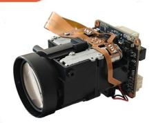
The IM50A01-10X is a cost-effective 5MP surveillance network camera module designed for both indoor and outdoor use. It features a 1/2.8" Sony IMX335 STARVIS sensor and is powered by the GOKE GK7205V300 SoC, equipped with 1Gb of RAM. In terms of extended I/O capabilities, it supports dual light source illumination, as well as microphone and speaker connections, enabling two-way audio and additional interfaces.
