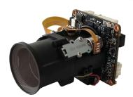
The IM50A01-5X is a cost-effective 5MP surveillance network camera module designed for both indoor and outdoor use. It features a 1/2.8" Sony IMX335 STARVIS sensor and is powered by the GOKE GK7205V300 SoC, equipped with 1Gb of RAM. In terms of extended I/O capabilities, it supports dual light source illumination, as well as microphone and speaker connections, enabling two-way audio and additional interfaces.
