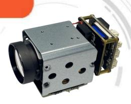
The IPA800Z10 4K Real-time lighting AI high-definition network camera module adopts upgraded H.265 encoding technology, and the environmentally friendly series brings efficient video compression capabilities. It can save bandwidth and storage space. Embedded web server, supporting internet exploration monitoring, configuration, and upgrade; Standard SDK (Linux, Windows), easy to integrate with other digital systems.
