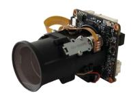
The IM20A03-4X is a cost-effective 2MP surveillance network camera module designed for both indoor and outdoor use. It features a 1/2.8" Sony IMX307 STARVIS sensor and is powered by the GOKE GK7205V300 SoC, equipped with 1Gb of RAM. In terms of extended I/O capabilities, it supports dual light source illumination, as well as microphone and speaker connections, enabling two-way audio and additional interfaces.
