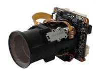
The IM50A01-4X is a cost-effective 5MP surveillance network camera module designed for both indoor and outdoor use. It features a 1/2.8" Sony IMX335 STARVIS sensor and is powered by the GOKE GK7205V300 SoC, equipped with 1Gb of RAM. In terms of extended I/O capabilities, it supports dual light source illumination, as well as microphone and speaker connections, enabling two-way audio and additional interfaces.
