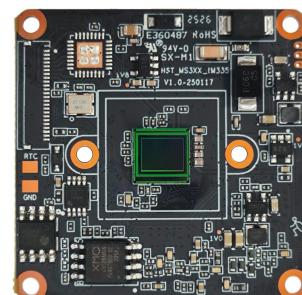
The IM50D01 is a cost-effective 5MP surveillance network camera module designed for both indoor and outdoor use. It features a 1/2.8" Sony IMX335 STARVIS sensor and is powered by the Sigmaster SSC377DE SoC, equipped with 1Gb of RAM. In terms of extended I/O capabilities, it supports dual light source illumination, as well as microphone and speaker connections, enabling two-way audio and additional interfaces.
